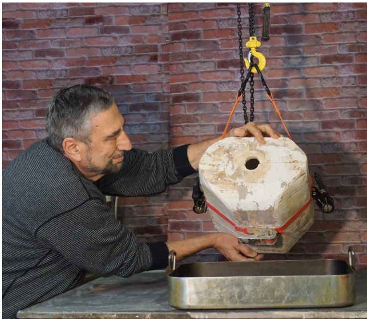
A Chain Puller – Lifting Heavy Molds Millburn, NJ, 2015
